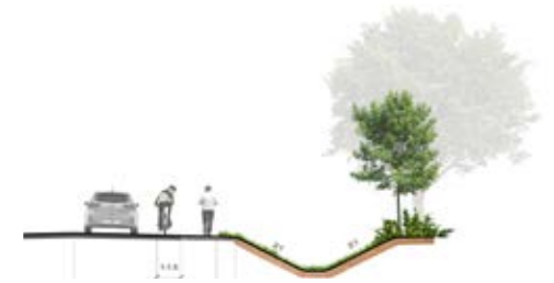
Cross section Rural Arterial with Paved Shoulder
